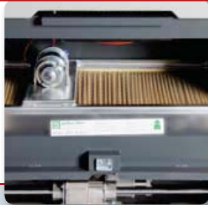
An electrical filter shaking system cleans the filter automatically every 5 minutes
